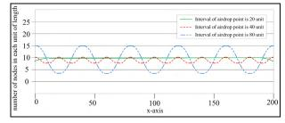
Figure 9. Density of sensors at different interval of airdrop point (100 sensors in total)
